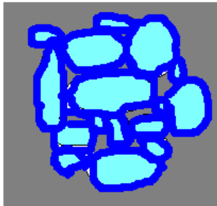
Particals covered with calcite bonding them together without significant loss of porosity
